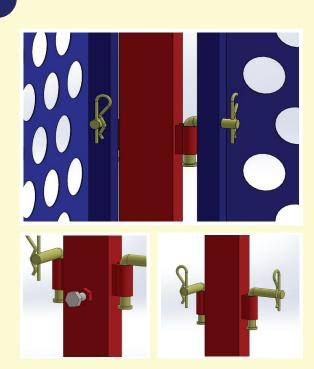
holes to enable connection of panels
