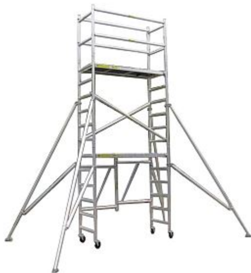
AR2.4 Standing high 3.25-3.75m, 0.73m wide, 2m long Access 5.5m high
